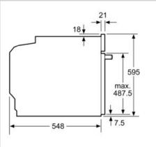
measurements in mm
